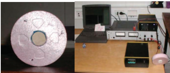
Figure 4: The left image shows the sample holder with a sample in the center. The right image shows the control units with the sample holder to the right.
